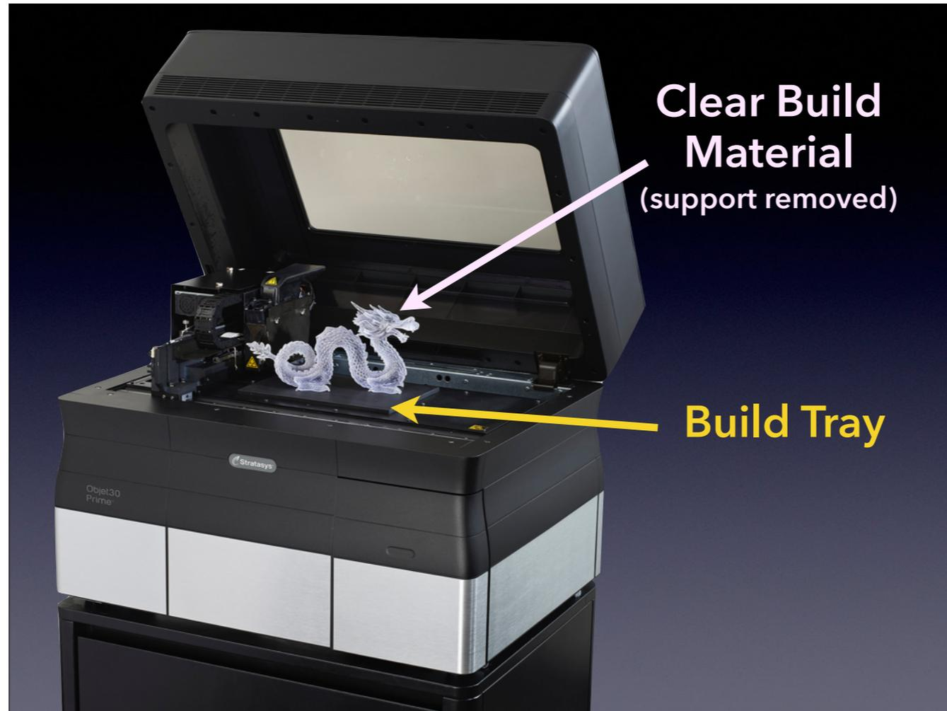
On this printer, the tray moves up and down. On many filament-based printers, the tray stays still and the head moves up and down.
